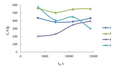
*Figure 4.* Dependence of the specific direct current capacity on the charge time at a current density of 2 mA/cm<sup>2</sup>
