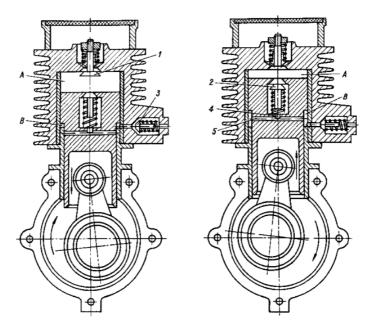
A - Cavity of the first stage; B - cavity of the second stage;
