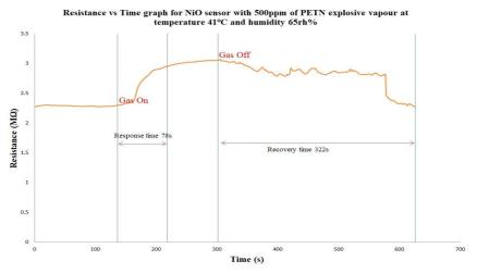
Figure 6. Switch behavior of NiO nanoparticles sensor with 500ppm of PETN explosive
