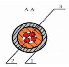
*Figure 3.* Heating element sample (1 - test sample; 2 - nichrome heater in a ceramic tube; 3 - copper tube)
