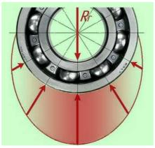
*Figure 2.* Scheme of the distribution of the radial load between the rolling elements in the bearing
