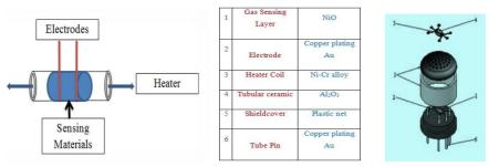
Figure.2 Constructed Tubular ceramic Al<sub>2</sub>O<sub>3</sub> substrate
