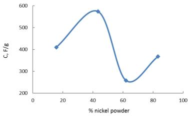
*Figure 5.* Dependence of the maximum specific capacitance of electrodes on the content of nickel powder in the composite coating
