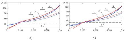
*Figure 2.* Static (1, 4) and dynamic (2, 3) suspension characteristics with a twochamber single-piston PHS at operating (a) and charging (b) temperatures: 1 - 5 - see fig. 1
