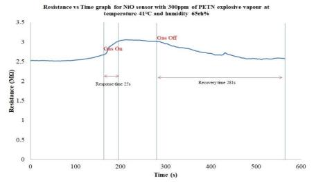
*Figure 5.* Switch behavior of NiO nanoparticles sensor with 300ppm of PETN explosive
