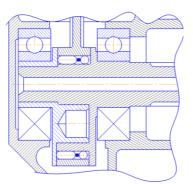
Figure 4. Local cut at the place of bearing replacement
