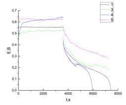
Figure 2 Charge-discharge characteristics of electrodes at a charge time of 3600 s and a current density of 2 mA/cm<sup>2</sup>
