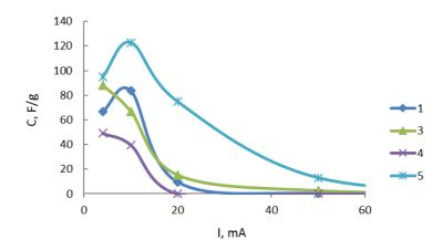
*Figure 3.* Dependence of the specific capacitance of the electrodes on the discharge current during charging for 300 s
