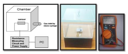
Figure 3. Explosive testing system chamber and multi-meter
